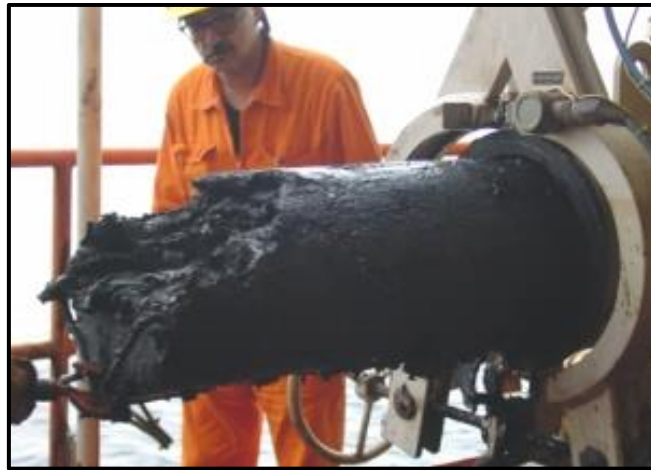
Figure 1. Asphaltene – Potential Pipeline Blockage [1]
