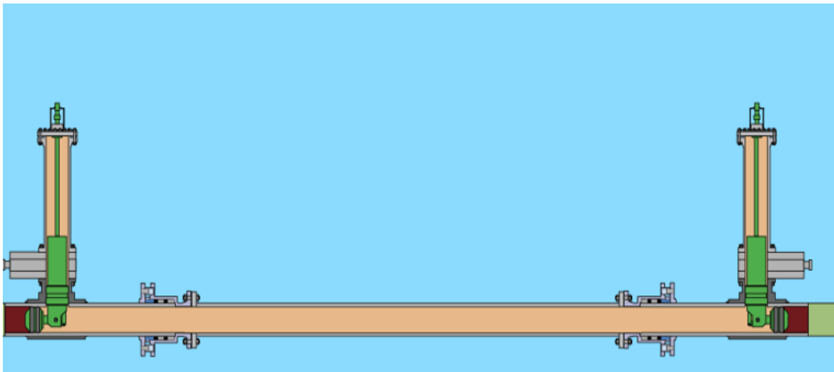
Figure 26. Replace pipeline section Leak test new connections against rear of BISEPS
