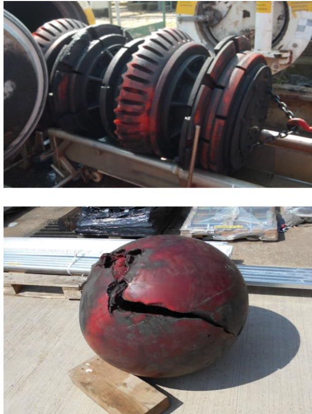
Figure 6: Recovered Damaged Sphere and Rescue Pig
