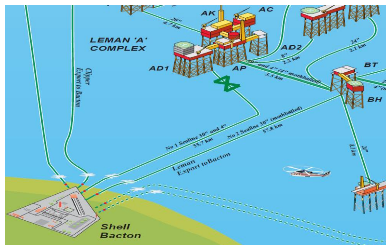
Figure 1: Leman – Bacton Pipeline System Overview
